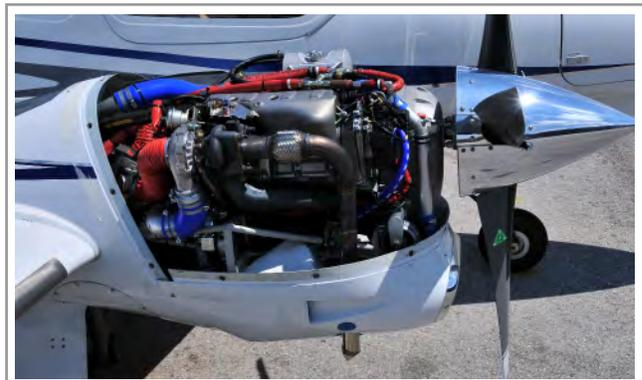
The DA42 NG utilizes two 170 hp turbo-diesel AE 300 engines.
