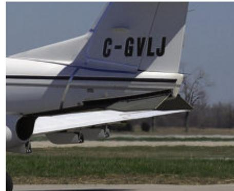
D-JET S/N001 taxiing out to flight test Ventral Strakes
