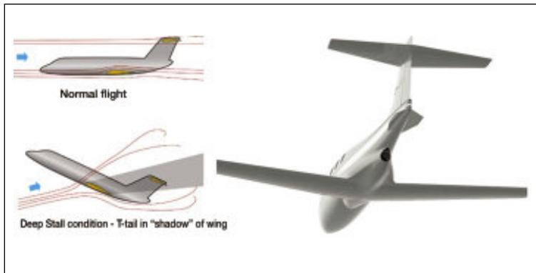
How they work. In a “Deep Stall” pitch control can be lost because the wash from the wing can blank the horizontal stabilizer and elevator. V-strakes are in clean air and will force the nose down until pitch authority is regained or prevent the high angle of attack to begin with.
