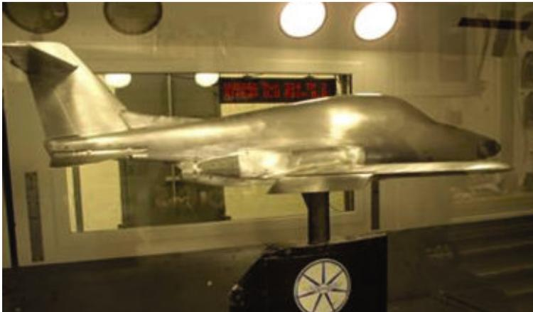
Optimizing planform and orientation angle in the windtunnel.
