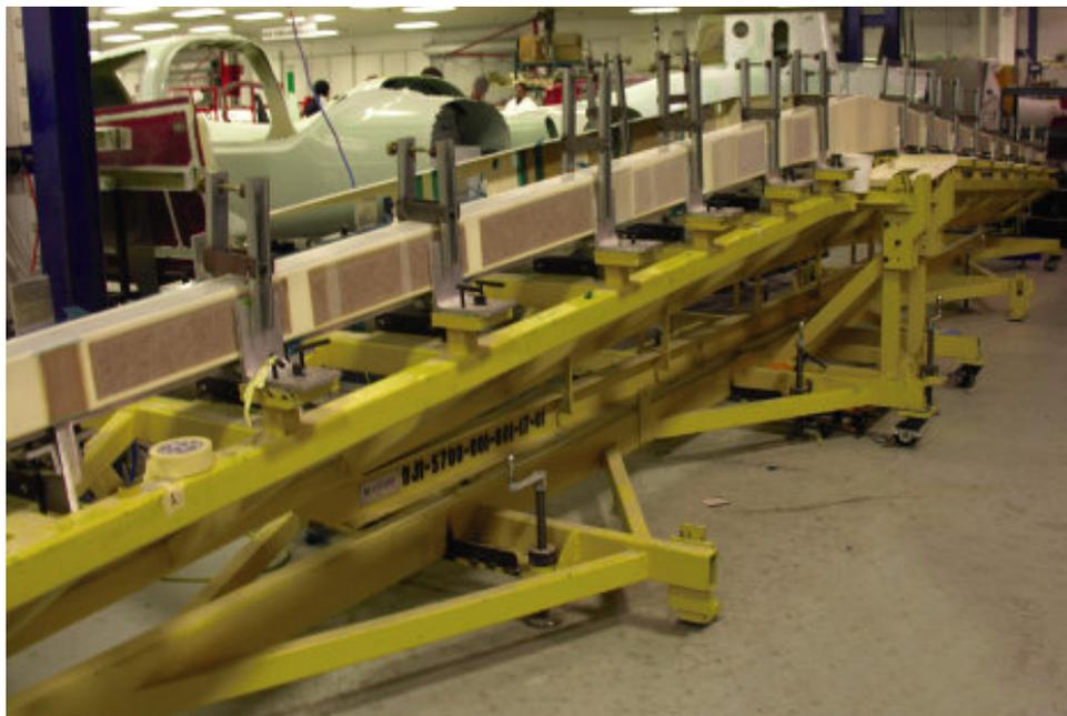
Wing assembly fixture with S/N003 wing spar
