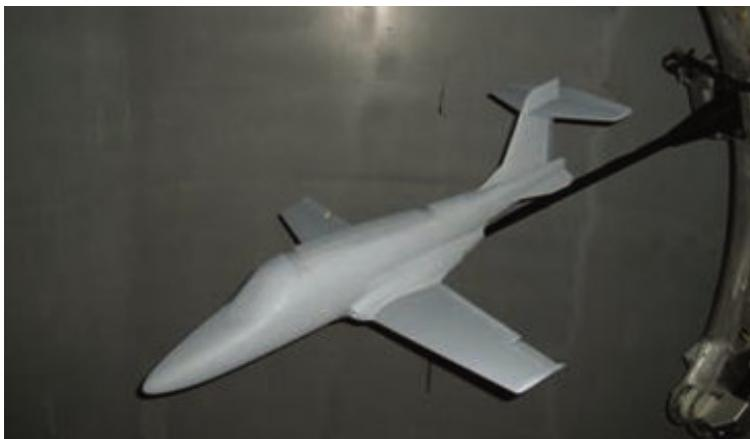
High Angle of Attack testing in Vertical Windtunnel. In this tunnel, the air flows from the bottom to the top.
