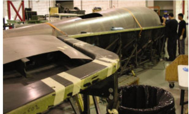
S/N003 fuselage shells being bonded in the mold
