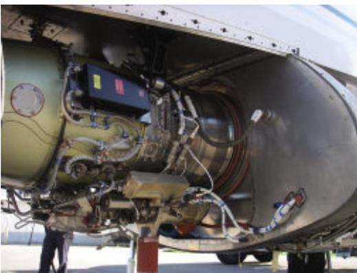
A picture is worth a thousand words: D-JET engine uncowled shows excellent accessibility of engine for maintenance
