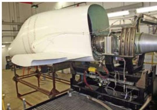
The FJ33 in an early D-JET inlet distortion test.
